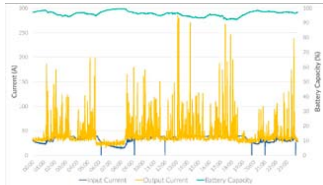
Figure 2. Performance metrics for the Enertainer at the AMC project on 8 July 2020, one of the busiest days for the tower crane on the project.
